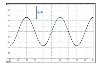
The RMS value, 6V, does not leap out as an obvious characteristic of this trace.
