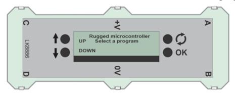
The LK8886 Micro ECU has six standard Locktronics legs that allow it to be inserted into the Locktronics base board.
