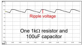
The traces for the circuits that use a 100μF capacitor do not show steady DC at all for the currents demanded.
